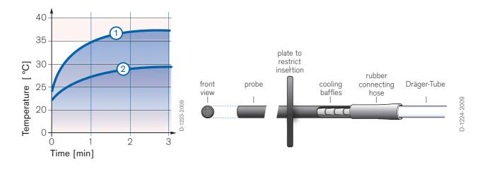
Cooling effect of the hot air probe gas temperature: 650 °C ambient temperature: 20 °C In 3 minutes 1 L of gas was drawn and the temperature in the tube rose according to the above curves (1) with one hot air probe (2) with two hot air probes Sketch of the hot air probe
